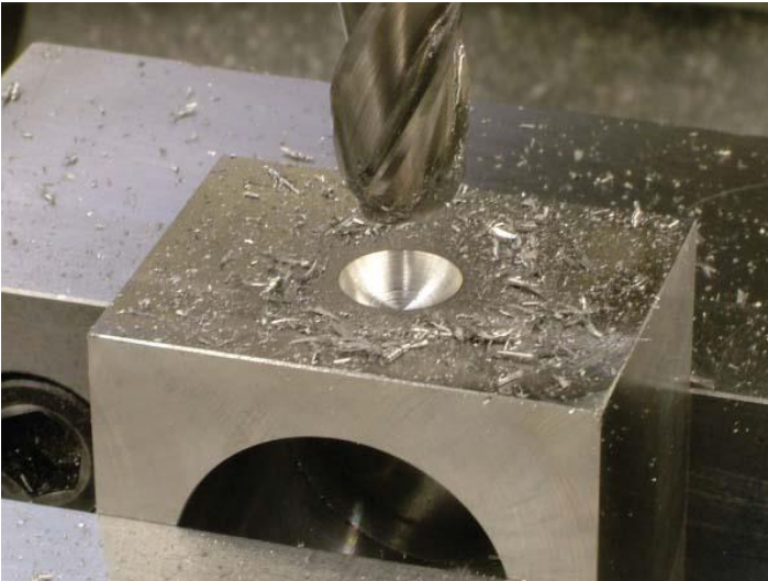
FIGURE 6.3.90 (A) Radius slots. (B) A spherical depression machined with a ball endmill.
