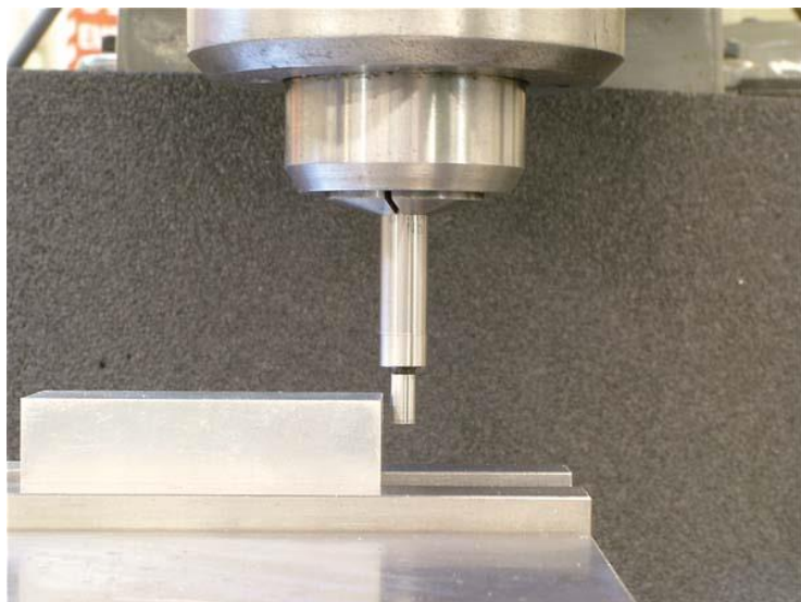
FIGURE 6.3.20 Positioning an edge finder near the edge of a workpiece.
