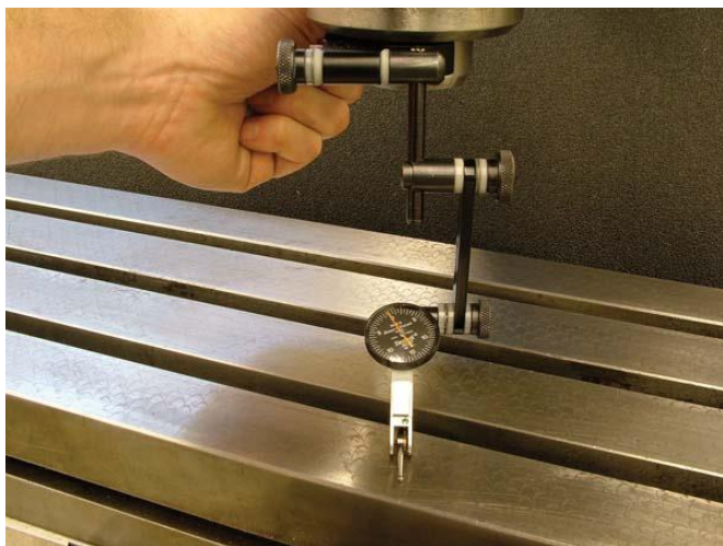
FIGURE 6.3.4 Using a dial indicator mounted on the spindle to “sweep” the table surface.
