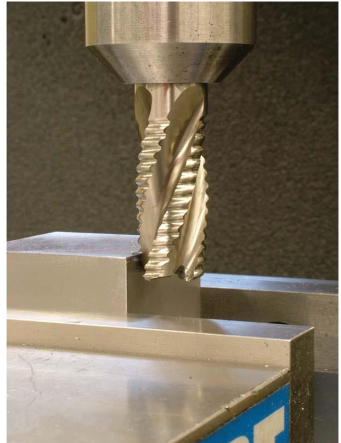
FIGURE 6.3.70 Touching off with a roughing endmill to set a reference for step width.
