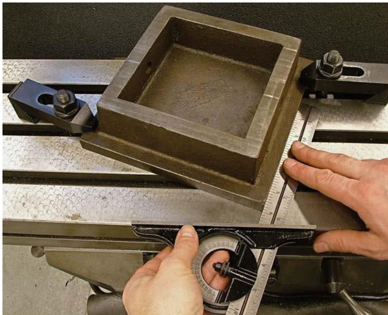
FIGURE 6.3.59 Aligning a large workpiece with a protractor using the edge of the machine table as a reference surface.
