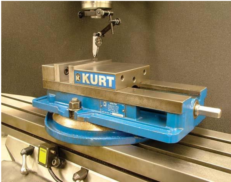
FIGURE 6.3.12 A vise can also be aligned with the saddle movement.
