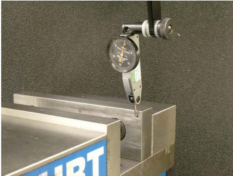
FIGURE 6.3.9 Positioning a dial indicator for aligning a vise with the table movement. Always indicate the solid jaw when aligning a vise.
