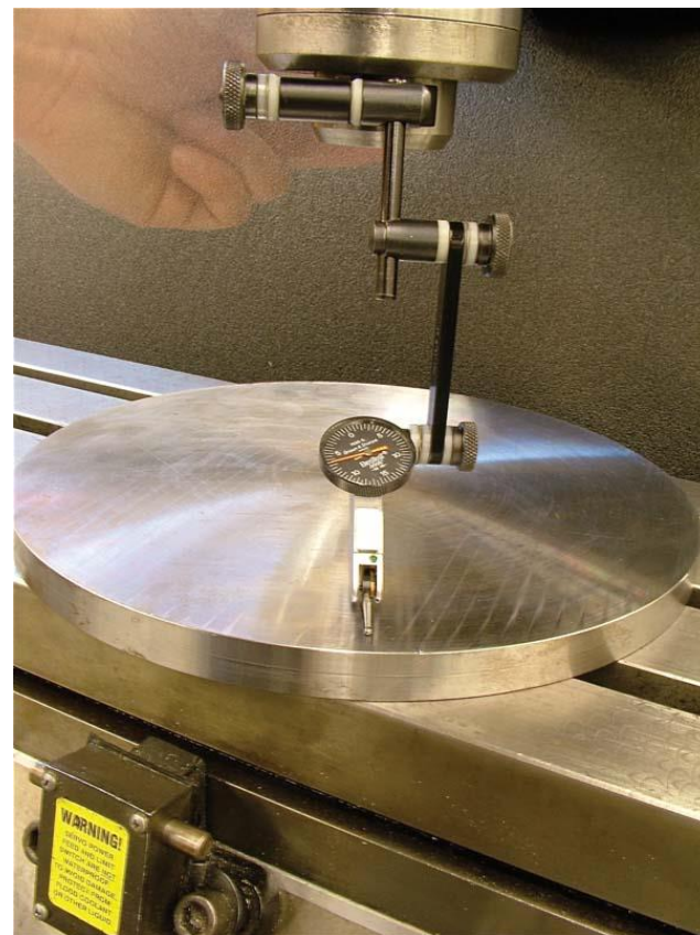
FIGURE 6.3.6 Using a dial indicator and flat disc to check the tram. © Cengage Learning 2012
