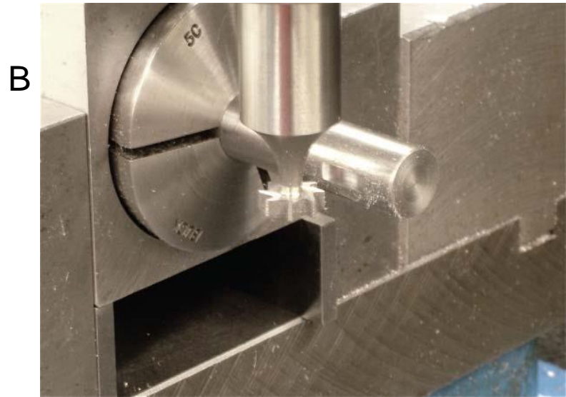
FIGURE 6.3.83 (A) Machining a woodruff keyseat. (B) The finished keyseat.
