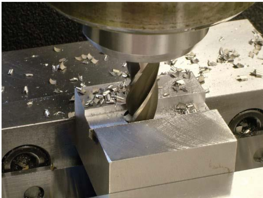
FIGURE 6.3.79 (A) Milling a through slot, and (B) a closed plain keyway. All images © Cengage Learning 2012
