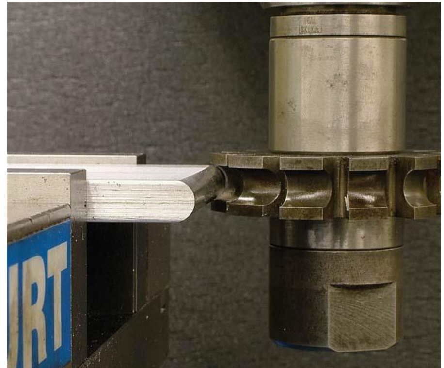
FIGURE 6.3.87 A full external radius machined by a stub-arbor-mounted concave milling cutter.
