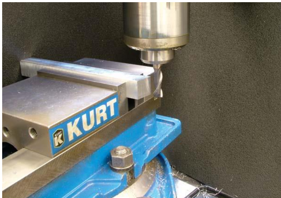
FIGURE 6.3.63 Milling an angular surface with the work held in a swivel-base vise.
