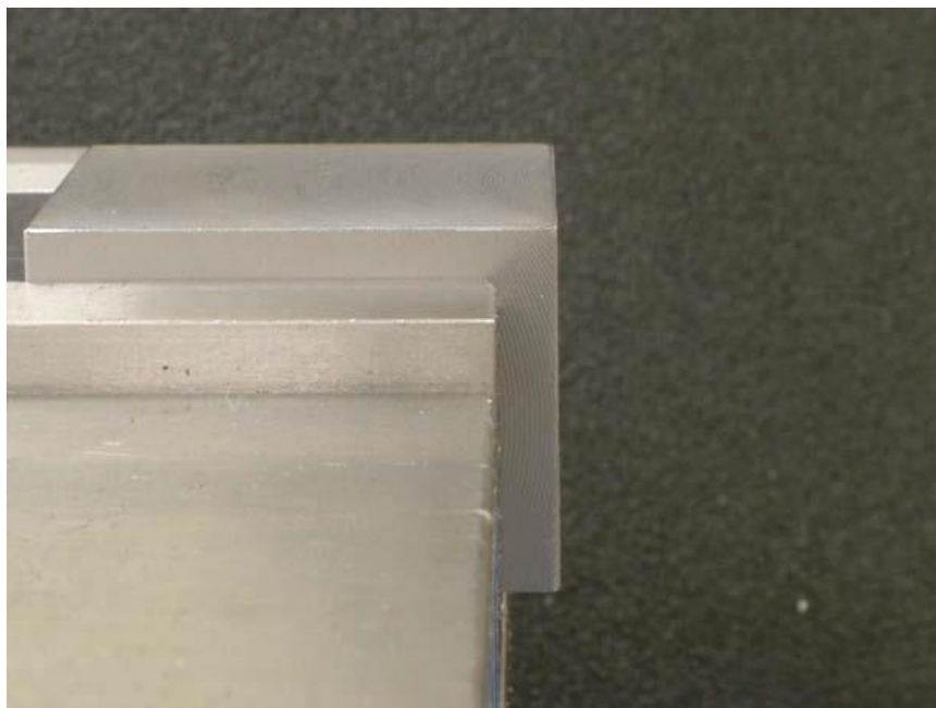
FIGURE 6.3.44 Side E can also be machined using an endmill by mounting the block in the vise with one end extended past the end of the vise jaws.
