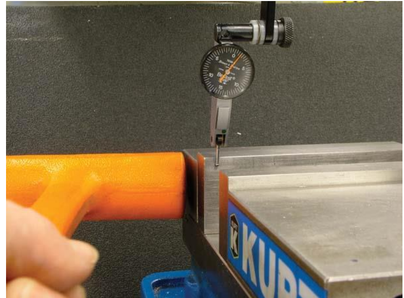
FIGURE 6.3.10 Using a dead blow hammer to tap the vise during alignment. Make adjustments until the TIR is 0.0005" or less. Recheck TIR after fully tightening the clamps.
