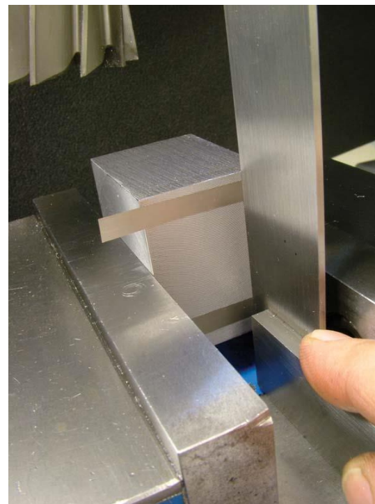
FIGURE 6.3.43 Using a solid square and feeler gages to position the block for machining Side E.
