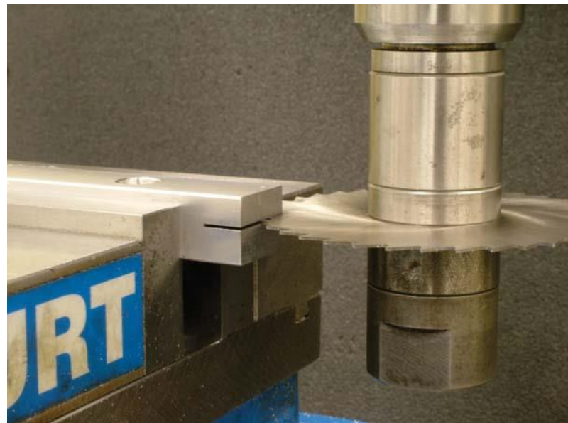
FIGURE 6.3.83 (A) Machining a woodruff keyseat. (B) The finished keyseat.
