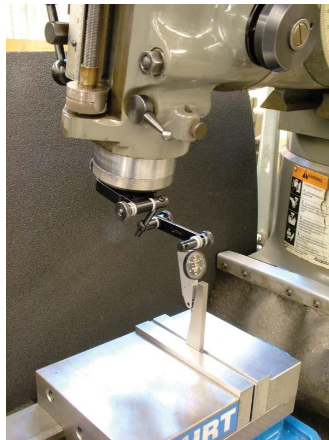
FIGURE 6.3.67 Indicating an angle block held in a vise by moving the quill. When the indicator reads “0” across the block, the angular setting is correct.
