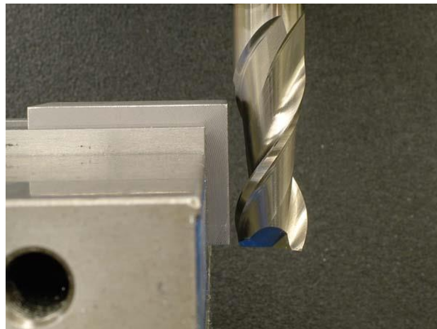
FIGURE 6.3.45 Position the endmill so the bottom extends past the bottom of the block. Be sure the flutes are long enough to span the entire surface to be milled.
