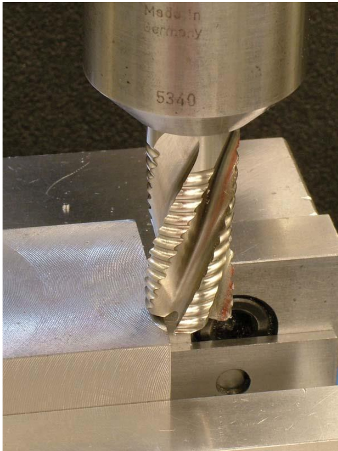
FIGURE 6.3.69 Touching off with a roughing endmill to set a reference for step depth.
