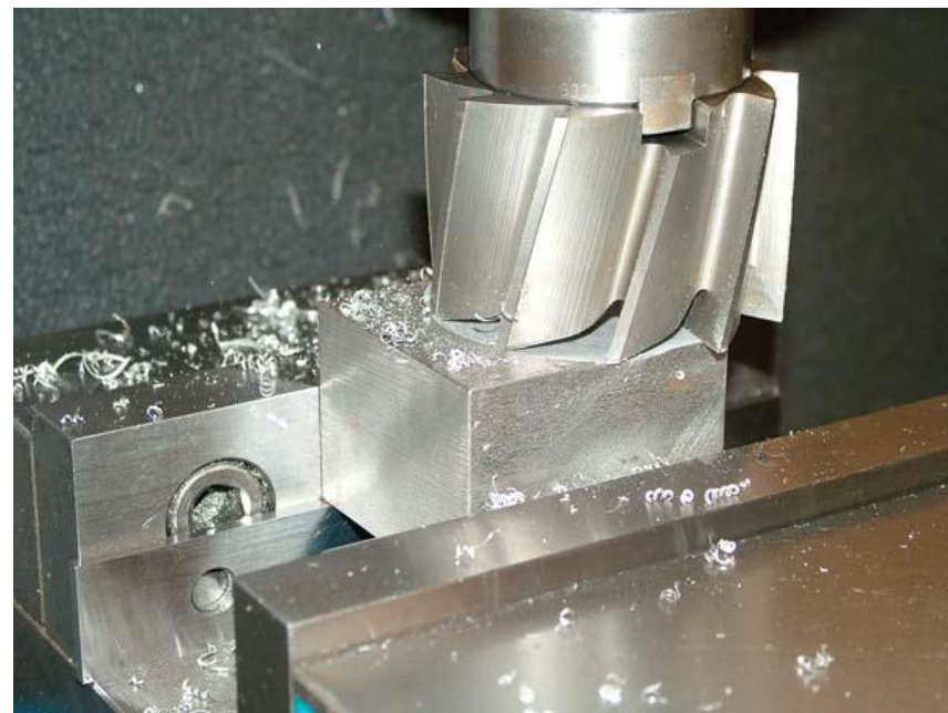
FIGURE 6.3.38 An HSS shell endmill facing the top surface of a block.
