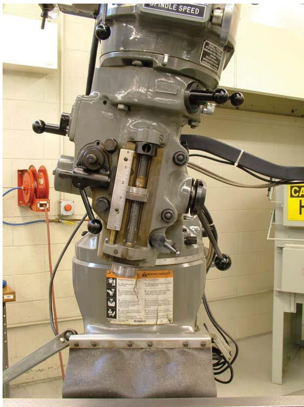
FIGURE 6.3.1 This tilted milling machine head must be trammed before machining square and parallel surfaces. © Cengage Learning 2012
