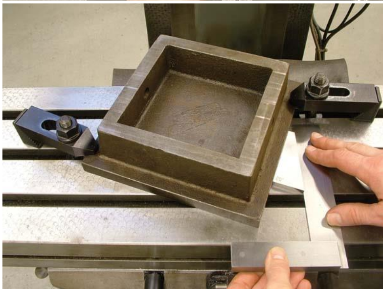
FIGURE 6.3.60 Positioning a large workpiece using an angle block and square. The square provides a reference surface relative to the table movement.
