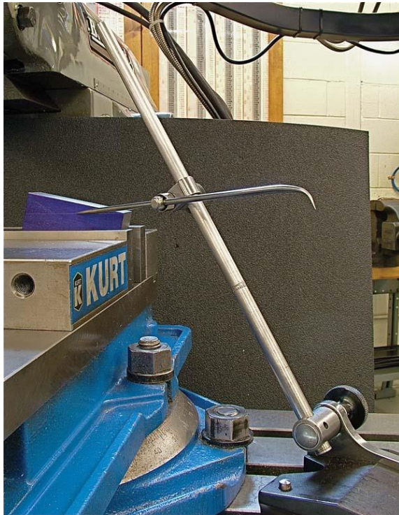
FIGURE 6.3.55 Positioning work to a layout line using a surface gage for milling an angular surface.
