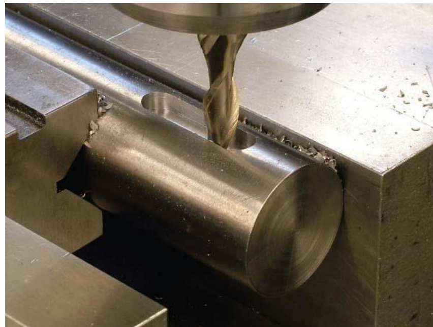
FIGURE 6.3.79 (A) Milling a through slot, and (B) a closed plain keyway. All images © Cengage Learning 2012
