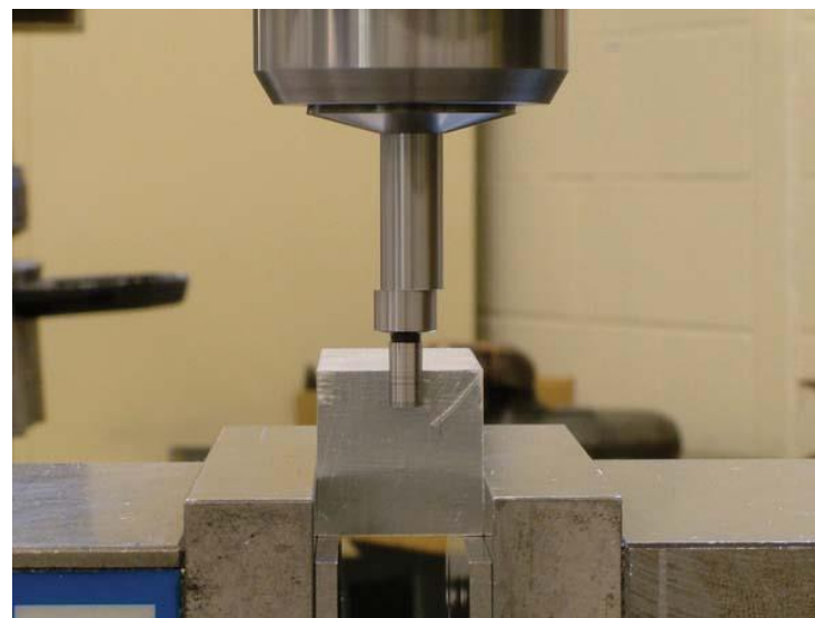
FIGURE 6.3.21 (A) When the tip of the edgefinder “kicks,” (B) the centerline of the spindle is one-half of the tip diameter from the part edge.
