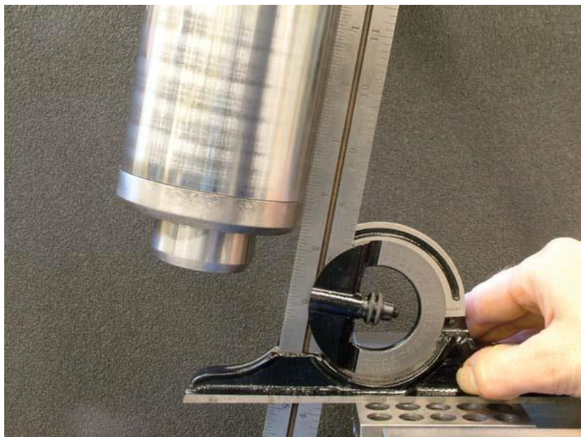
FIGURE 6.3.66 A protractor can be held against the quill to check the angular setting of the mill head. Hold the protractor head against the solid vise jaw so that the blade is in line with the direction of the angular movement.
